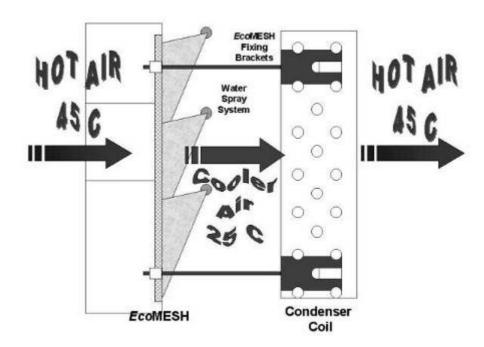
It is estimated that this additional adiabatic ambient cooling before the condenser coil should provide an increased capacity of  $14 \sim 15\%$  in comparison with the original chiller design. This corresponds to  $\sim 26\%$  energy efficiency improvement.
